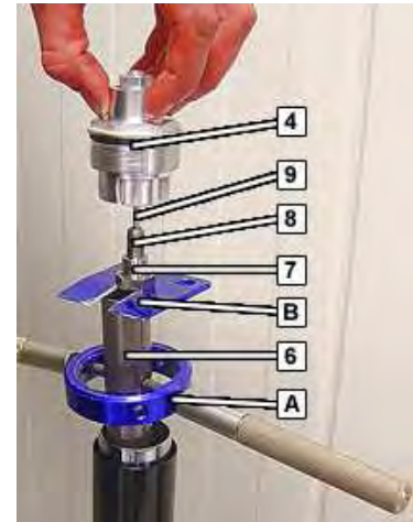
Fork with reversed preload
